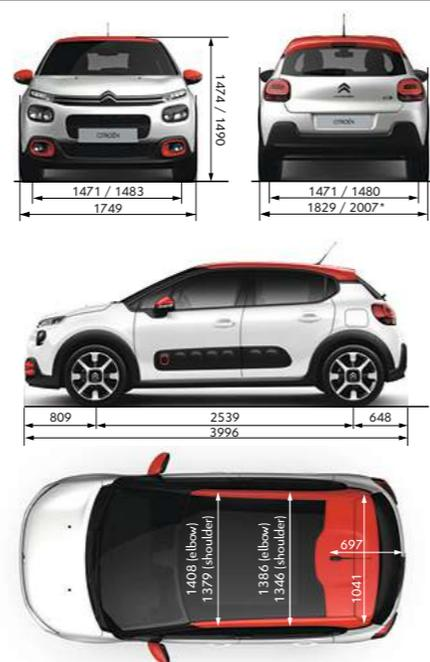
\* Vehicle width/width with slide mirrors out. All measurements are in millimetres.
