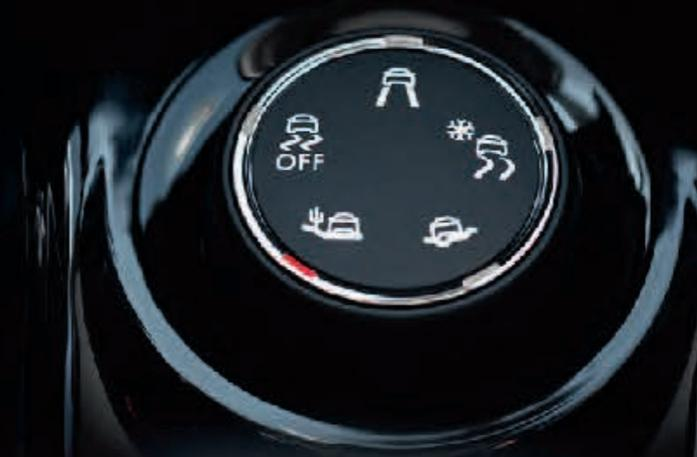
Grip Control® optimises traction in low-grip conditions. It adapts to different terrain by acting on the front wheels, using electronic components already present on the vehicle meaning that it adds no extra weight and therefore no excessive fuel consumption, unlike a traditional 4x4. Standard from Allure\* level, on both manual and automatic versions, it is coupled with 17" alloy wheels.
